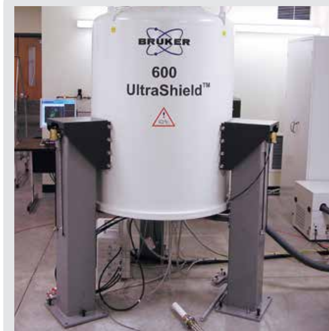
600 MHz NMR on PAL18 gimbal air springs
