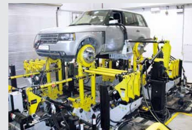
Chassis dynamometer on a vibration-isolated foundation
