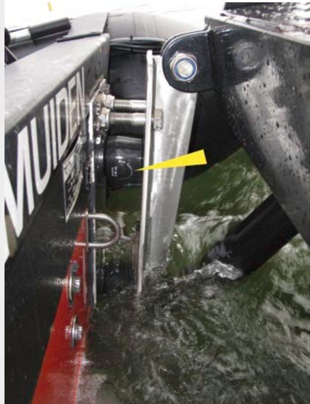
Seawater-resistant, robust TUBUS profile dampers made of co-polyester elastomer allow boats and crew to dock safely
