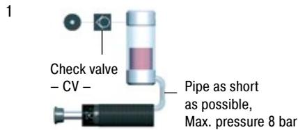
Piston rod returns immediately to extended position when load moves away. Operation without main air supply possible for short periods.
