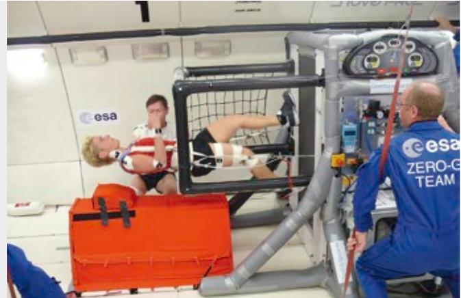
TUBUS are used to protect a fitness machine in zero gravity
