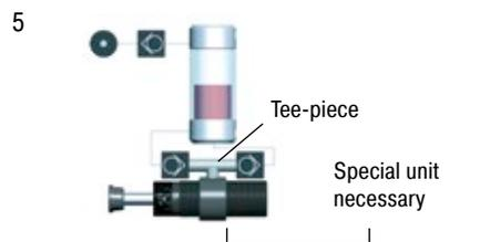
Oil recirculation circuit for extreme high cycle rates. Warm oil is positively circulated through air/oil tank for increased heat dissipation.
