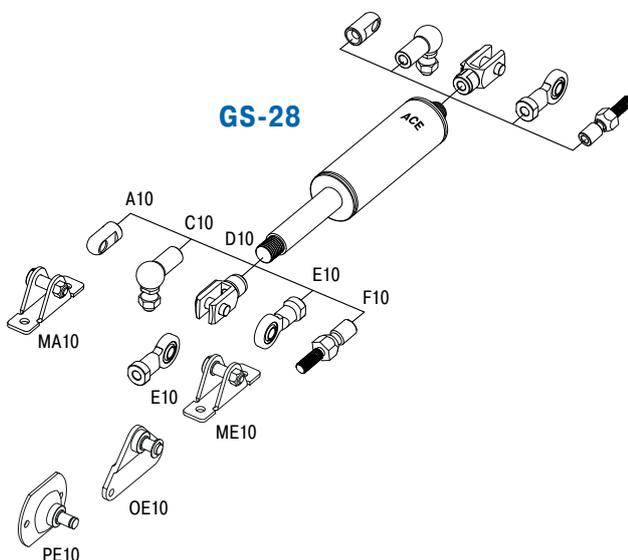
Valve Technology, Force range 500 N to 5,000 N (compressed up to 7,450 N)
