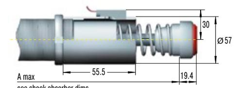
inc. Proximity Switch and Poly Button with elastomer insert
