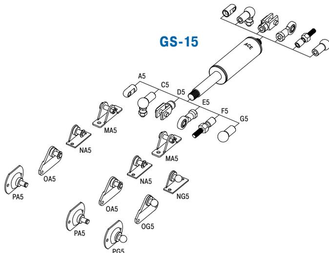
Valve Technology, Force range 50 N to 700 N (compressed up to 970 N)
