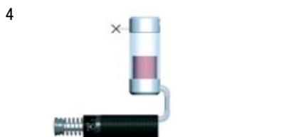
Spring return with air/oil tank. No air supply connected. Note: Will extend return time.
