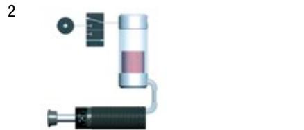
Return stroke may be sequenced by pneumatic valve at any desired time. No return force until valve energised.
