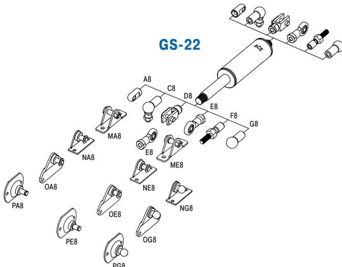
Valve Technology, Force range 150 N to 2,500 N (compressed up to 4,175 N)
