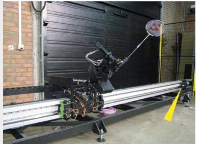
A variety of different dampers are used to slow the rapid movements of a badminton robot
