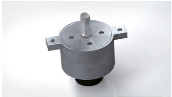
The damping direction of the adjustable FYT-H1 and FYN-H1 can be right, left or two-sided rotation. During each reverse movement of the unilateral decelerating versions there is a certain return damping torque that depends on the size. The brakes have a particularly robust zinc die-cast body and shafts made of steel. ACE rotary dampers are maintenance-free and ready-to-install.
