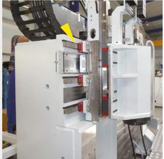
ACE clamping and safety elements maintain a rock-solid hold on the axes in special lathes and secure the predetermined positions both horizontally and vertically
