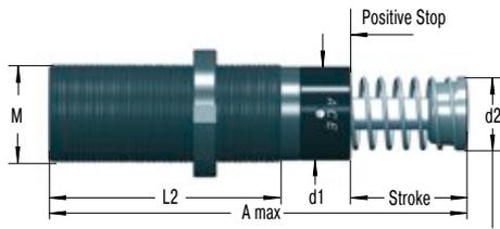
150 mm stroke model does not include stop collar.
