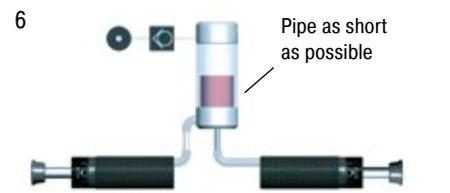
Oil recirculation circuit for extreme high cycle rates. Warm oil is positively circulated through air/oil tank for increased heat dissipation.
