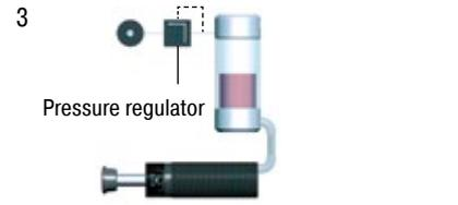
Return force can be adjusted by pressure regulator. Ensure safe minimum pressure to return shock absorber.
