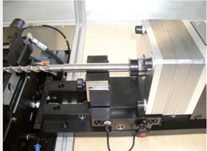
ACE clamping elements assist in the production of drilling tools: the LOCKED-P system clamps and at the same time absorbs the opposing forces of the joining process without difficulty
